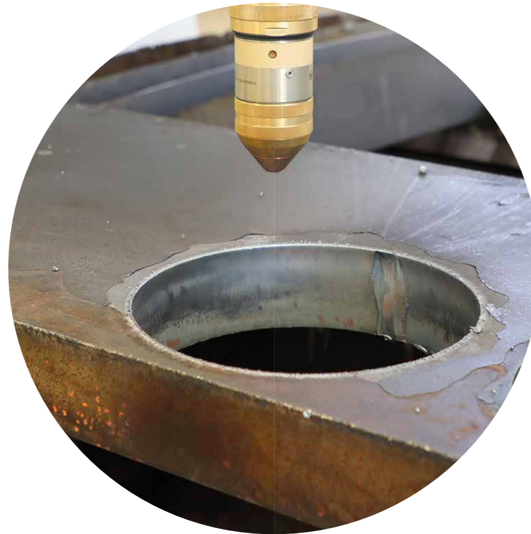
Q 1500 Cutting range mild steel 0.5 - 60 mm piercing up to 50 mm
